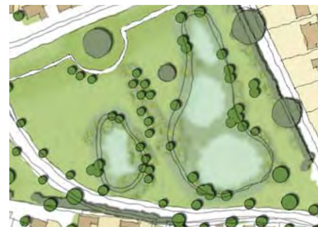
Attenuation Ponds to lowest point of site on eastern boundary.
